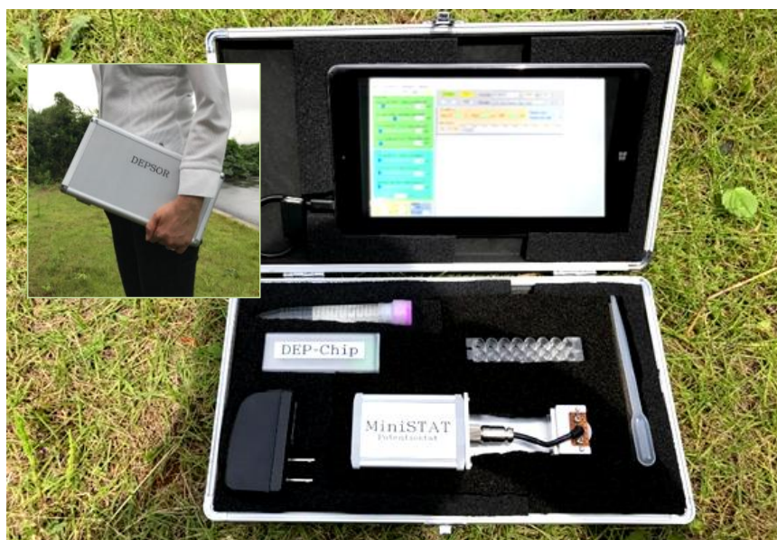
Figure 2. Photographs of handheld DEPSOR unit and components including palm-sized USB-powered potentiostat, Screen-printed disposable electrode chips, and PC tablet with semi-automatic software for on-site voltammetric analysis.
